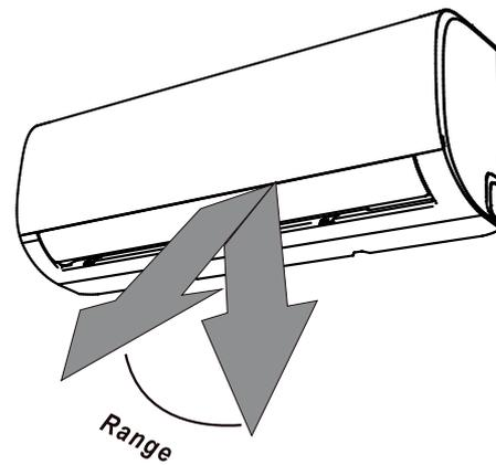
**!** Caution: Do not keep louver at too vertical an angle for long periods of time. This can cause water condensation to drip on your furnishings.
