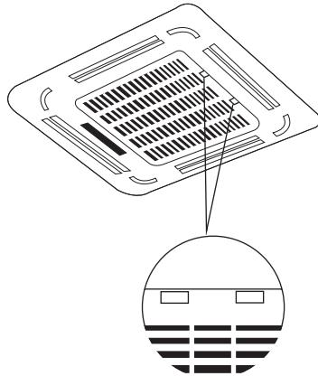
Adjust the panel by turning it to the arrowed direction so that the ceiling opening is completely covered.
