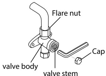
11. Using hexagonal wrench, fully open both the high pressure and low pressure valves.
