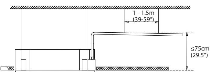
**NOTE:** When connecting multiple drainpipes, install the pipes as illustrated in the following Figure.
