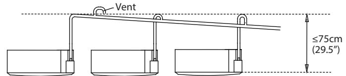
Pass the drain hose through the wall hole. Make sure the water drains to a safe location where it will not cause water damage or a slipping hazard.
