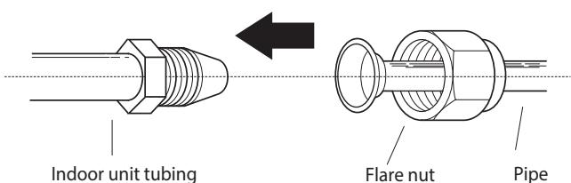
3. Tighten the flare nut as tightly as possible by hand.
