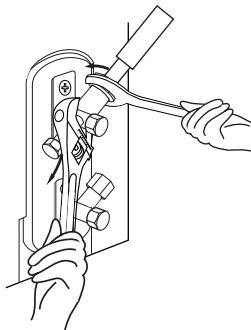
8. Remove the flaring tool and flare form, then inspect the end of the pipe for cracks and even flaring.
