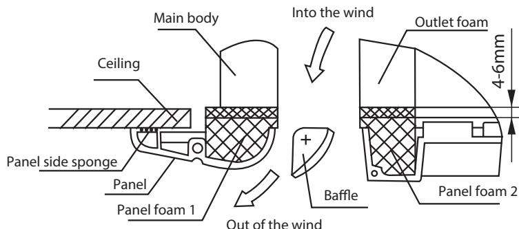
**NOTE:** If the height of the indoor unit needs to be adjusted, you can do so through the openings at the panel's four corners. Make sure that the internal wiring and drainpipe are not affected by this adjustment.
