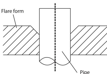
6. Place flaring tool onto the form.
