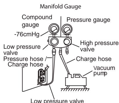
6. Close the Low Pressure side of the manifold gauge, and turn off the vacuum pump.
