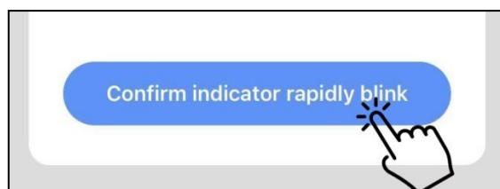
Notes: when the icon of set flashes quickly, it mean the controller is in the Wi-Fi mode. When it flashes slowly, it means the controller is connecting with the App. During the connection, if the icon of set is extinguished, it means the App connection with the unit is finished.
