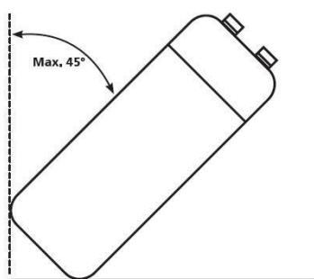
**⚠ ATTENTION: DUE TO THE HIGH CENTER OF GRAVITY, LOW OVERTURNING MOMENT,
