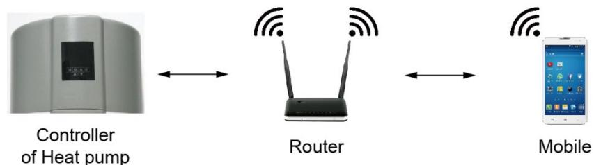
Power on the heat pump unit, and keep pressing the timer button and the increase button at the same time for 5 seconds. The SET
