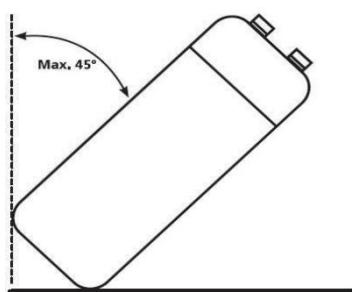
**⚠ ATTENTION: DUE TO THE HIGH CENTER OF GRAVITY, LOW OVERTURNING MOMENT, THE UNIT MUST BE SECURED AGAINST TIPPING OVER.**
