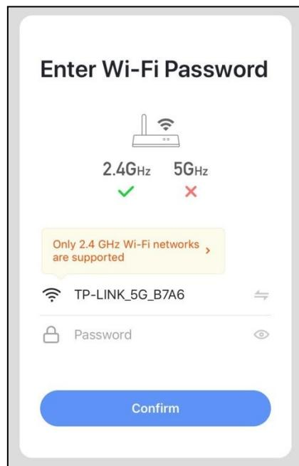
After click "Confirm", the Wi-Fi module, mobile device and Wi-Fi router begin to be connected. Finish the connecting, and the interface will be skipped to the next interface.
