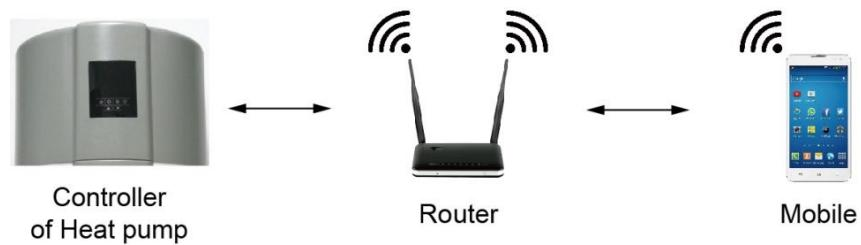
Power on the heat pump unit, and keep pressing the timer button and the increase button at the same time for 5 seconds. The SET
